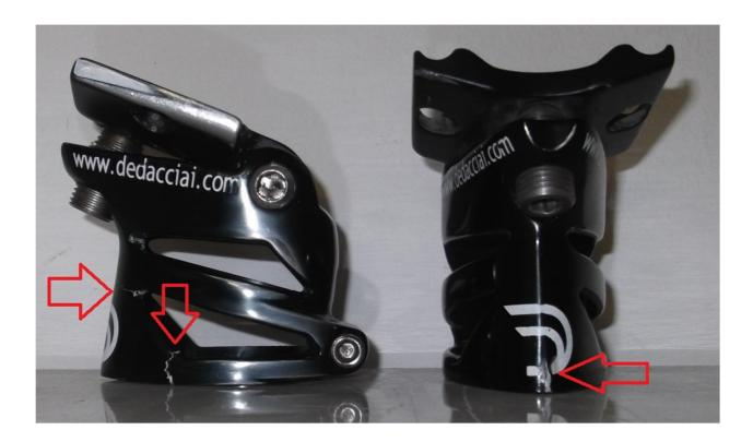
If you notice the listed cracks on the back and on lateral body we kindly invite you to quit the bicycle utilization as the KING PIN can crack and eventually break during normal use, that may cause the rider to lose control, fall and suffer potentially serious injuries.
